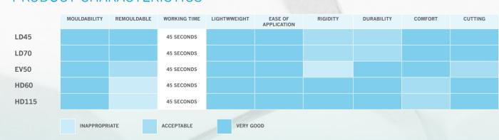
Guide 'working times' are based on 6mm thick material for HDPE grades and 12mm thick material for other grades. The product range is constantly being updated; new colours, new densities or more specialist foam grades. Full information on request.
