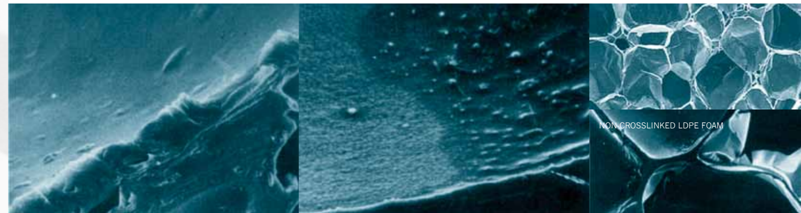
CROSSLINKED AND CHEMICALLY EXPANDED LDPE FOAM
